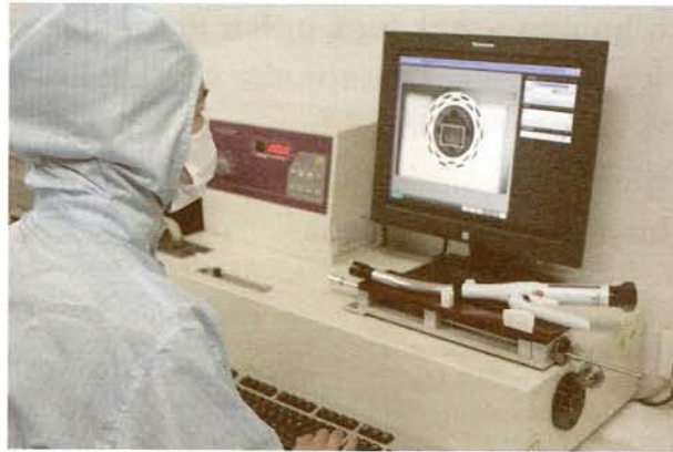
Inspection of presence and integrity of staples in staple housing at Frankenman's cleanroom facility
